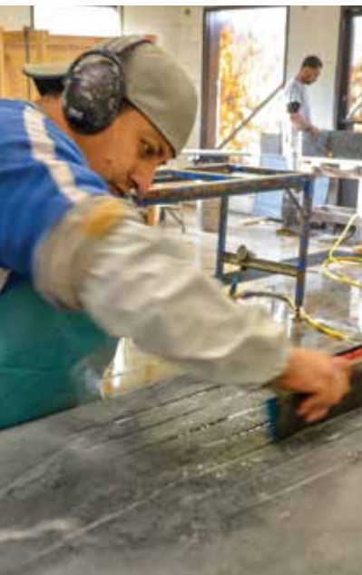
TOP (left) Leonardo Ribeiro, production manager and shop foreman, lowers a stone slab into position on the cutting bed. (right) A monitor shows both worker and CNC machine exactly where cuts are to be made on the slab. ABOVE The sharp edges of a grooved countertop are hand-sanded by Angel Paguay. INSET A native of Brazil, Roger Teixeira has been in the soapstone business for 25 years.
